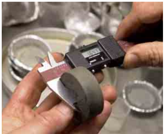
Figure 4.8 Soil specimen from the Bothnia Line dismantled from the oedometer ring subsequent to test. Re-measuring with the purpose of checking the total deformation
