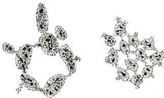
Figure 2.24 Undisturbed clay, schematic illustrated patterns. On the left-hand side, particle structure of marine clay and on the right-hand side lacustrine clay, modified after Pusch (1978)
