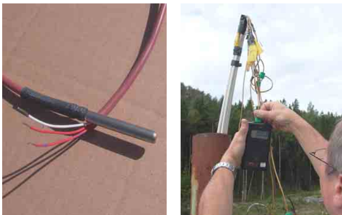
Figure 5.6 On the left-hand side temperature sensor, type Pt100. On the right-hand side; manual reading of the soil temperatures at different depths
