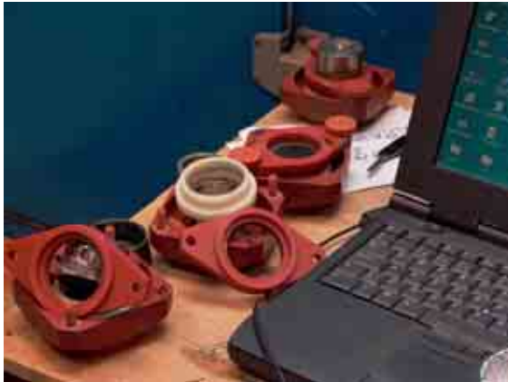
Figure 4.5 The oedometer equipment, enumeration from the centre; oedometer ring (white), below; top porous stone collar (red), in the top; stamp (steel), ultimately, the bottom porous stone collar, i.e. the fixed ring container (red)
