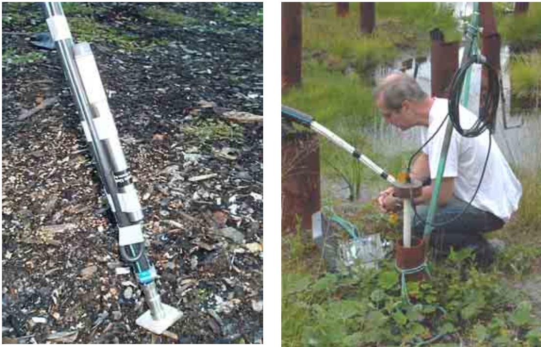
Figure 5.9 On the left-hand side; piezometer mounted on the conduit at the ground level gauge. On the right-hand side; manual reading the vibrating wire piezometer at ground surface
