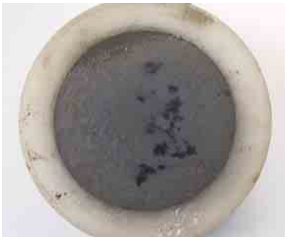
Figure 4.7 Soil specimen from the Bothnia Line fitted in the oedometer ring, before the test
